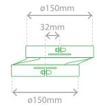
Air duct offset adapter included (inside dimensions)
